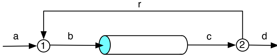
Figure 1. Schematic representation of the recycle PFR system of Example 31.1.
