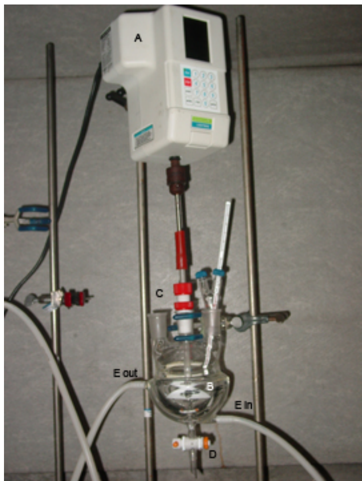
Figure 11.1. A simple round-bottomed flask that can be used as a perfectly mixed batch reactor. (In this photograph, the agitator, B, appears to be flipped upside down.)
